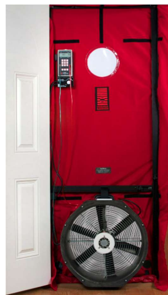
Blower door installed and ready for testing.
