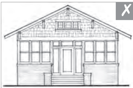
Existing Condition: Craftsman style house with an enclosed porch.
