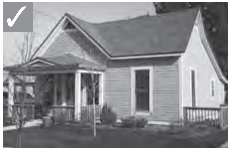
The porch on the left has experienced an inappropriate alteration; enclosed railing. Compare it with its “rehab” in the photo to the right.
