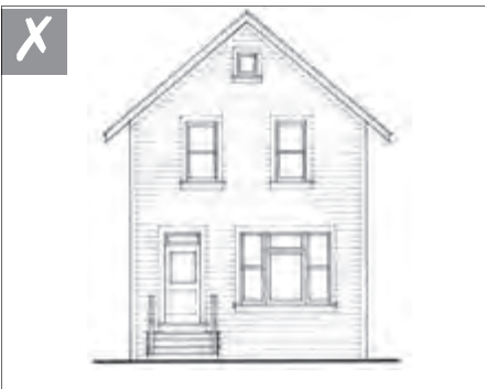
Existing Condition: A folk or vernacular style house with the original porch removed.
