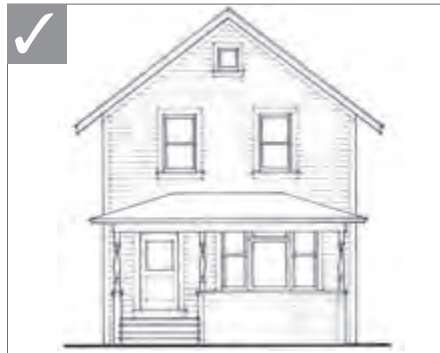
Preferred Approach, when historical documentation is available: A folk or vernacular style house with a replacement porch designed similar to that seen historically.
